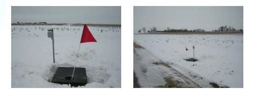
For *overland runoff*, a weir is installed to measure flow volume and allow for sample collection.
